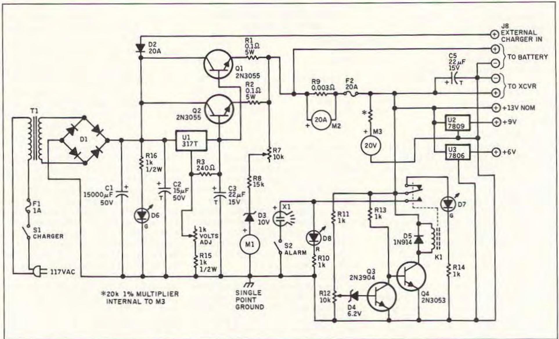
Figure 1. Backup battery monitor/charger/alarm schematic diagram.
